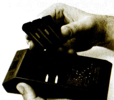
5. Insert the new battery pack so that its contacts face the calculator and contact is made with the battery connectors.
