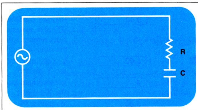
**Example 3:** Engineer Tobias Slothrop has determined that in the RC circuit shown above, the total impedance is 77.8 ohms and voltage lags current by  $36.5^\circ$ . What are the values of resistance  $R$  and capacitive reactance  $X_c$  in the circuit?
