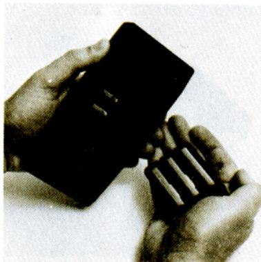
4. See if the battery connector springs have been inadvertently flattened inward. If so, bend them out and try the battery again.
