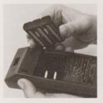
5. Insert the new battery pack so that its contacts face the calculator and contact is made with the battery connectors.
