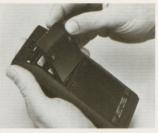
**6.** Insert the bottom of the battery door behind the retaining groove and close the door.
