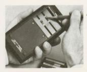
4. See if the battery connector springs on the calculator have been inadvertently flattened inward. If so, bend them out and try the battery again.
