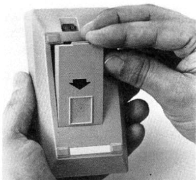
4. Insert the new battery pack in the direction of the arrow. Slant the leading edge of the pack into the edge of the doorway.
