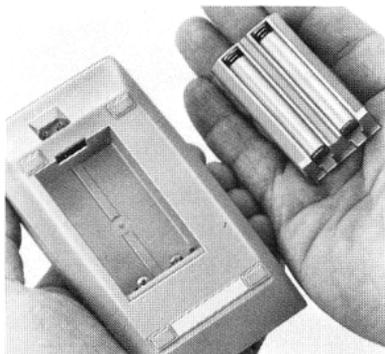
3. When the key on the battery pack becomes visible, lever that end of the pack up and permit the battery pack to fall into the palm of your hand.
