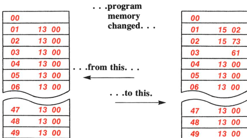
The illustration on the left shows program memory immediately after pressing **f** **PRGM** in PRGM mode or turning the HP-25 ON. The illustration on the right shows program memory after recording the three-step example program.
