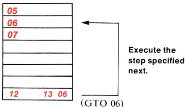
When recording an unconditional branch always follow the **GTO** key with two digit keys to designate the step number. For instance, to branch to step 6 the program instruction must be **GTO** **0** **6**.
