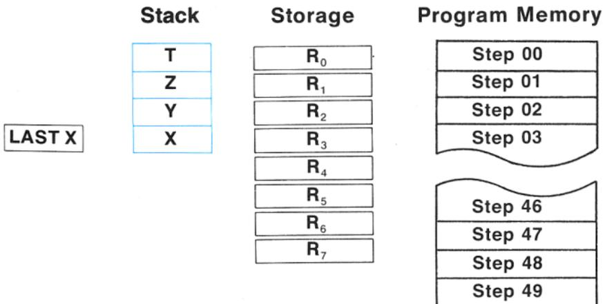
As you can see, the program memory for the HP-25 is separate from the four stack registers, the LAST X register, and the eight storage registers.
