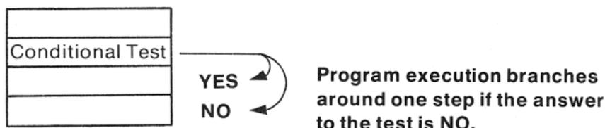
The eight different conditionals in your HP-25 are shown here. In each case, the tests are made on the 10-digit numbers and two-digit exponents actually stored in the stack registers, not on the displayed values.
