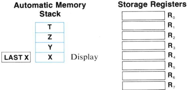
The addresses of the storage registers are indicated by number keys **0** through **7**, as shown above.
