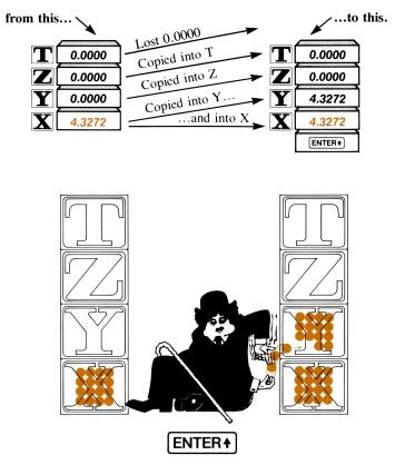
The number in the displayed X-register has been copied into Y. Numbers in Y and Z have also been pushed up into the Z- and T-registers, respectively. The number in T has been lost off the top of the stack. This process will be more apparent when different numbers are in all four stack registers.
